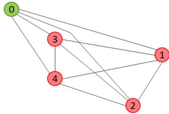
*Figure 1 The 5 node graph to be routed. Node 0 is the depot: the start and end point of the route.*
