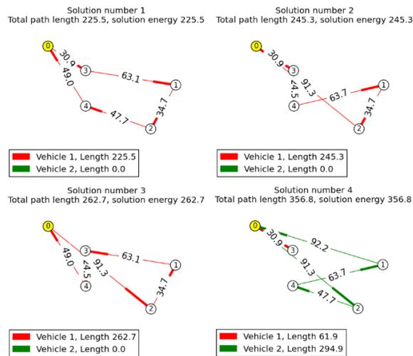
*Figure 2 The four best results from running the problem on the D-Wave Two. The thickened end of the edge-lines indicates where the vehicle starts from on each leg of its journey.*
